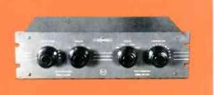
116F-1 PROGRAM EQUALIZER . . . provides complete facilities for controlling the frequency response of program and communication circuits. Since this unit has an insertion loss of 30 db, the Collins 6R Isolation Amplifier in association returns the level to normal, plus gain if desired.
