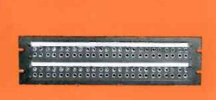
TYPE 265D JACK PANELS . . . provide connections for test purposes or for terminating program lines and order wires. Lines, amplifiers, microphones, equalizers, and other audio equipment can be speedily interchanged for maintenance or emergency operation. These jack panels mount in standard 19-inch racks. Regularly supplied with Collins 360 1010 00 jack.
