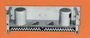
**117N-2 REPEAT COIL PANEL**... is a complete assembly including chassis, terminal board, and dust cover, but less repeat coils. This unit will accommodate four Thordarson type repeat coils with an R-4 case. Fifty terminals on the board make connections to external equipment. The Dust cover is held on by two convenient Dzus fasteners.
