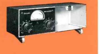
**60H TWO CHANNEL REMOTE MIXER** . . . is a two-position, low-level mixer to be used in conjunction with the Collins 212Y Remote Amplifier. It consists of a mixer chassis in a cabinet which has an opening for the insertion of the 212Y Amplifier. The 212Y slides into the 60H mixer case exactly as it does into its own case.
