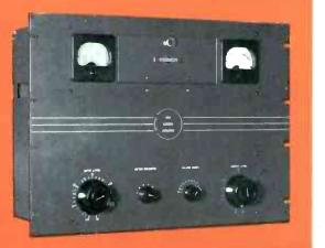
**26W-1 LIMITING AMPLIFIER** . . . is recommended for use in any AM, FM or TV installation to control the amplitude of audio. Limiting prevents overmodulation and accompanying distortion, permits a higher average modulation level.
