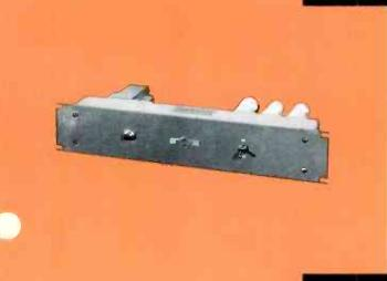
**409T-3 POWER SUPPLY** . . . rack mounted on a 3l/2'' panel. Connections are made to a covered terminal board at the rear. Any one of the output voltages and currents listed below is made available by changing two resistors supplied in a kit.
