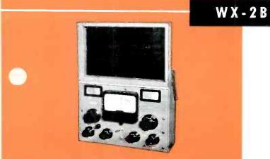
DISTORTION AND NOISE METER . . , measures distortion, noise, and hum level in audio frequency circuits and is continuously adjustable in frequency over the audio range. Measurements as follows: fundamental frequencies, 50 to 15,000 cps; noise and hum measurements, 30 to 45,000 cps; distortion values, as low as 0.1%.
