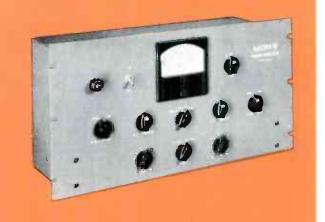
ANDREW 40-C PHASE MONITOR . . . facilitates adjustment and maintenance of broadcast directional antenna arrays. Phase Angles are indicated directly in degrees on a single meter, permitting immediate observation of the effects of small antenna system adjustments. Relative amplitude of antenna currents can be quickly determined with the ration appearing on a special ratio scale.
